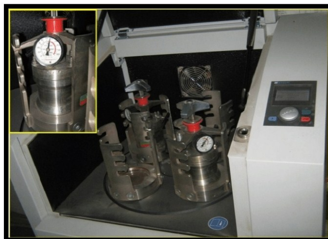
Figure 1: Planetary ball mill (RETSCH PM 400)
