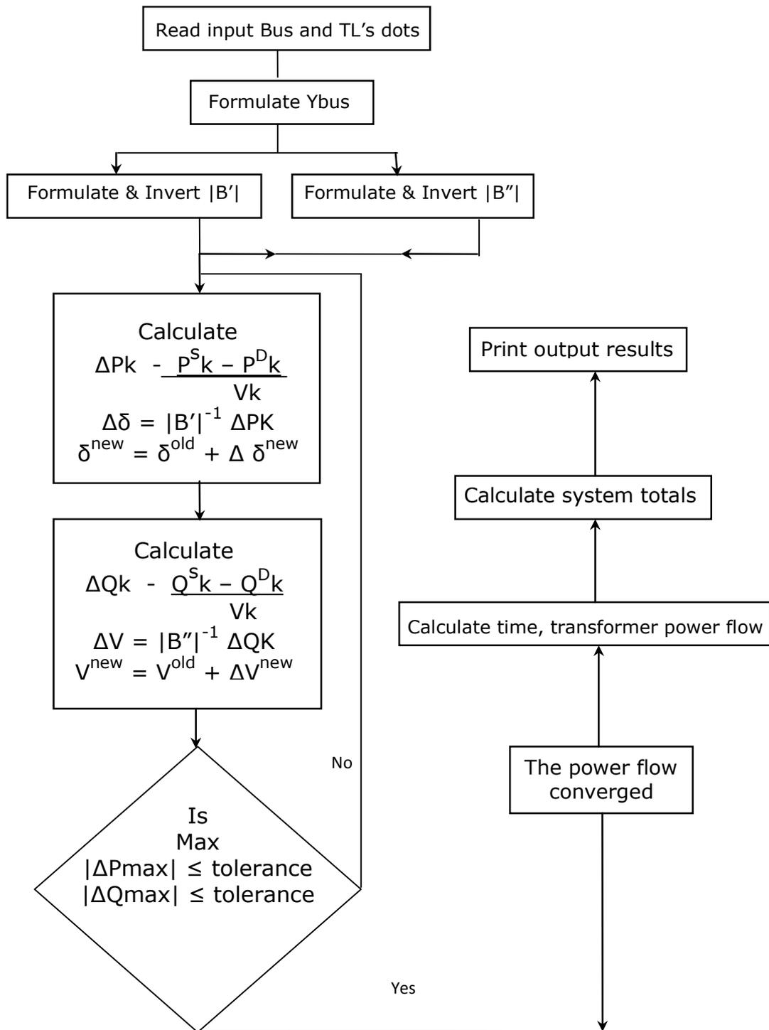
**Fig 1:** The flow chart for a fast decoupled power flow programme
