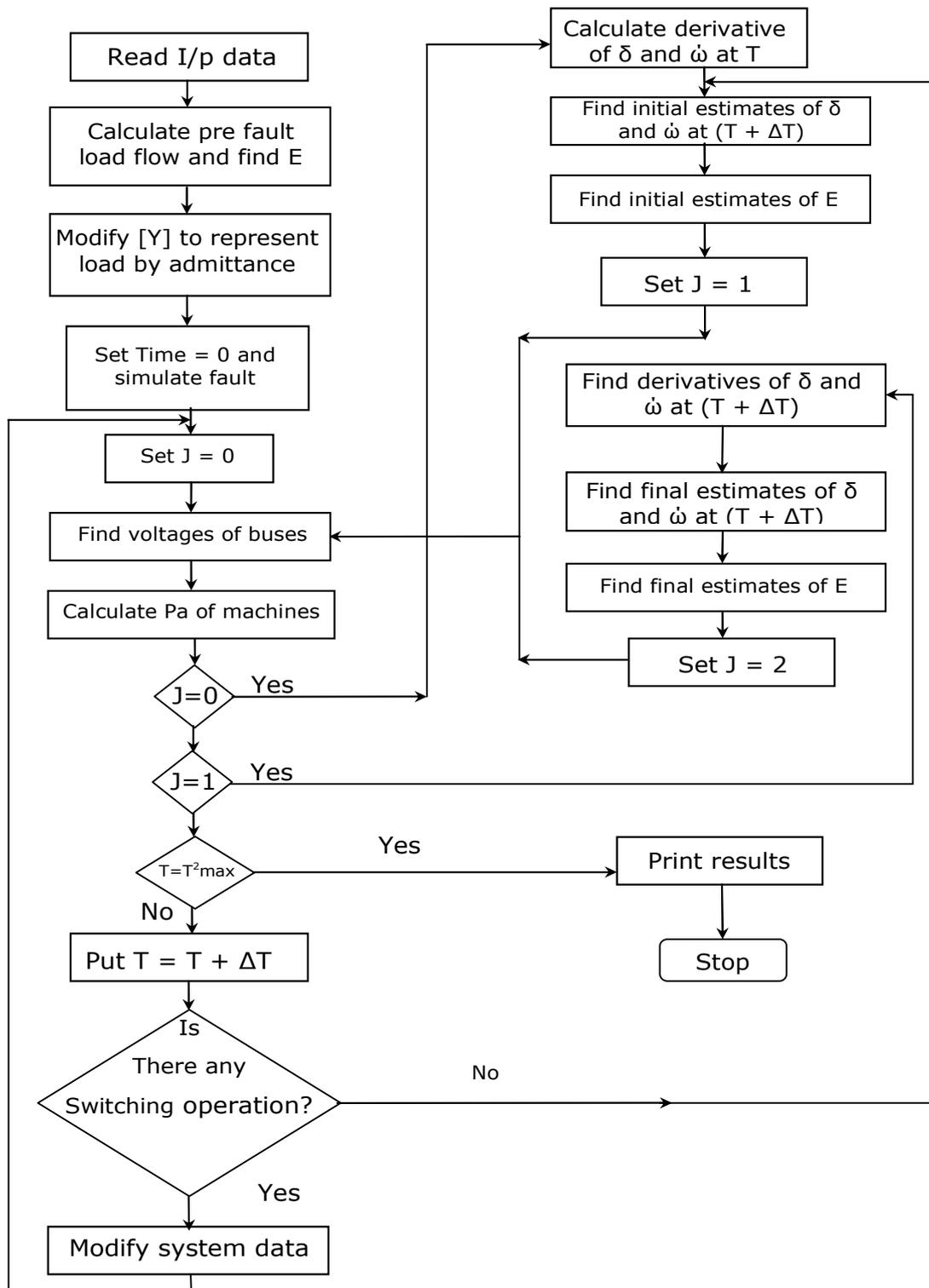
**Fig 2:** Flow chart of transient stability study using modified Euler's method
