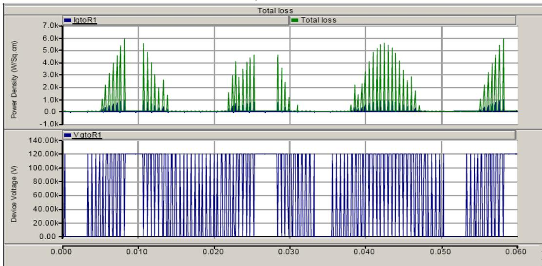
**Figure 1:** Loss profile for SiC GTO (300K)
