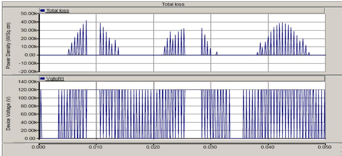
**Figure 6:** Loss profile for Si GTO (423 K)
