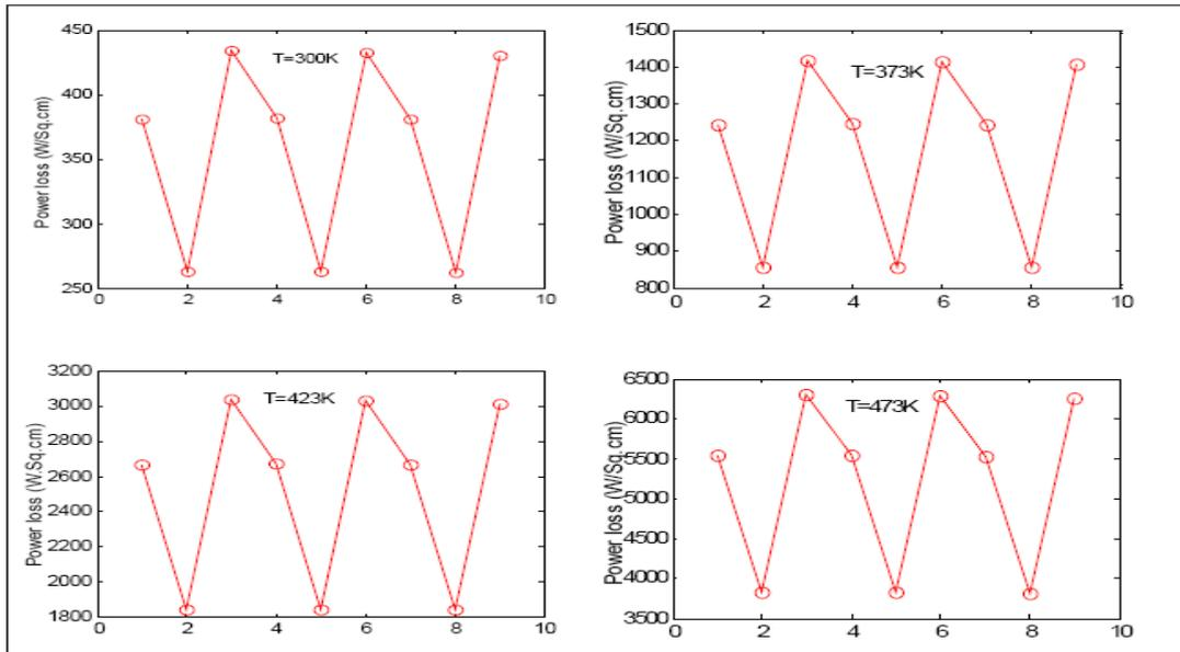
**Figure 8:** Cyclic power loss plots for Si 5KV, 200 A/cm<sup>2</sup> GTO
