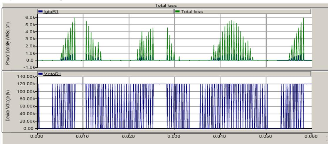
**Figure 5:** Loss profile for Si GTO (300 K)
