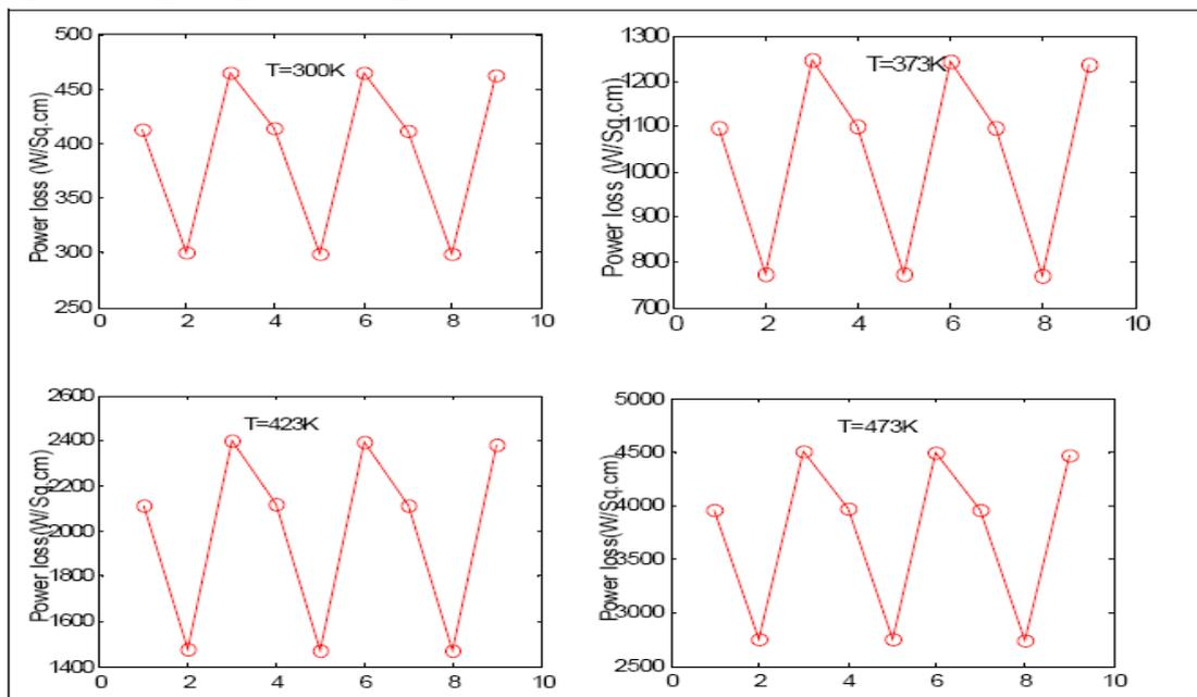
**Figure 9:** Cyclic power loss plots for SiC 20KV, 200 A/cm<sup>2</sup> GTO
