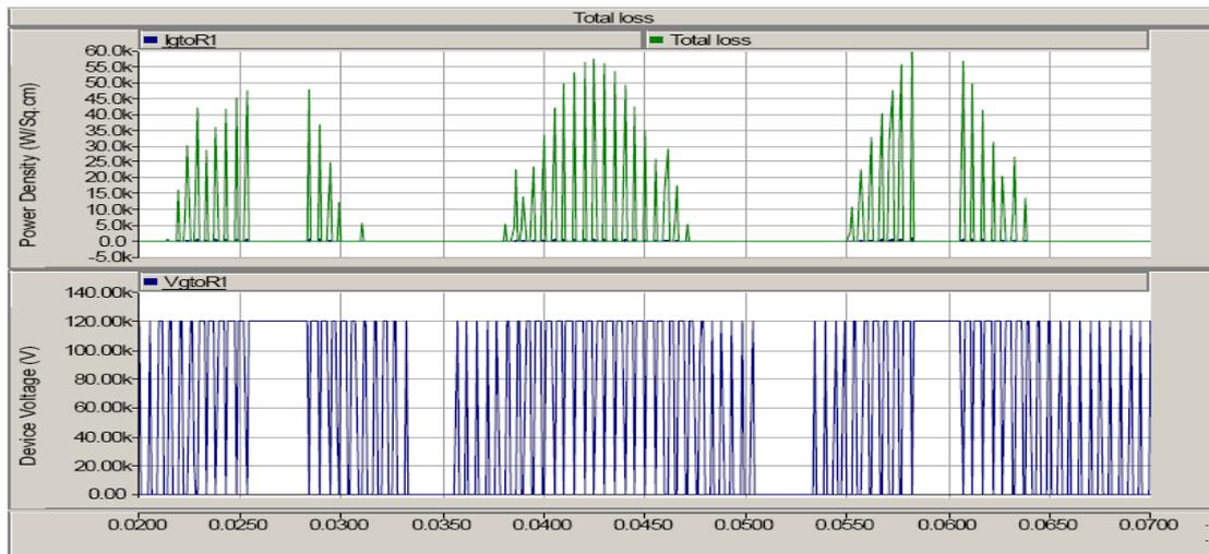
**Figure 3:** Loss profile for SiC GTO (473 K)
