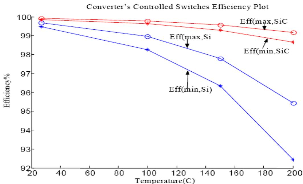
Figure 10: Converter's Controlled Switches efficiency plot
