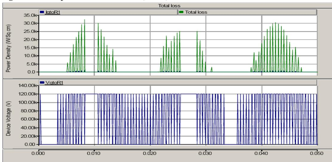
**Figure 2:** Loss profile for SiC GTO (423 K)
