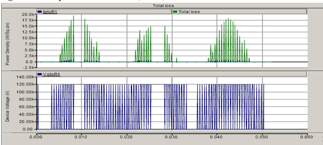
**Figure 4:** Loss profile for Si GTO (373 K)
