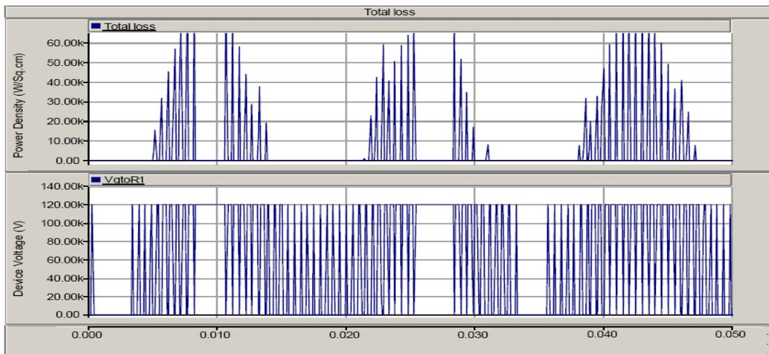
**Figure 7:** Loss profile for Si GTO (473 K)
